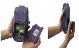
Insert the two plastic teeth in the gaps on the i7910 case, place the battery into the cavity and push it. Press the battery handle until a click is heard.
